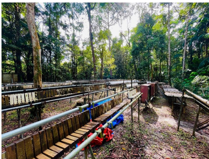
Figure 2. L-joints exposed in Malaysia. Photo: DTI.
